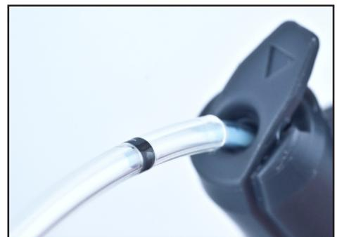
**The Visible Strain Relief Marker indicates the catheter is not fully inserted**
